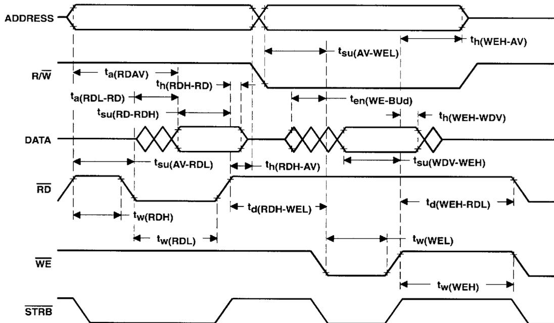
NOTE A: All timings are for 0 wait states. However, external writes always require two cycles to prevent external bus conflicts. The above diagram illustrates a one-cycle read and a two-cycle write and is not drawn to scale. All external writes immediately preceded by an external read or immediately followed by an external read require three machine cycles.
