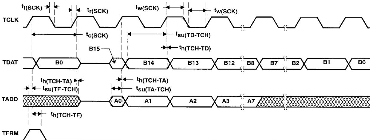
Figure 17. Serial-Port Receive Timing in TDM Mode
