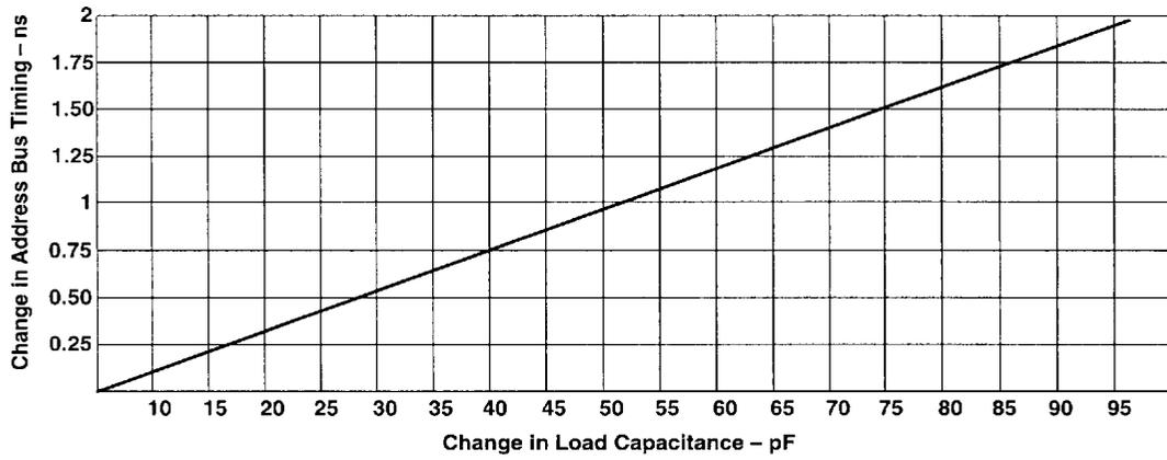
Figure 8. Address Bus Timing Variation With Load Capacitance
