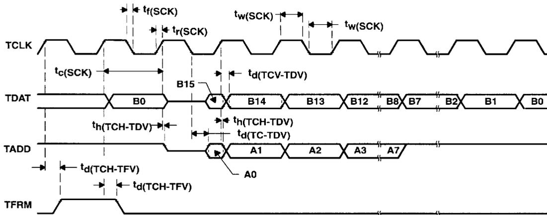
Figure 18. Serial-Port Transmit Timing in TDM Mode
