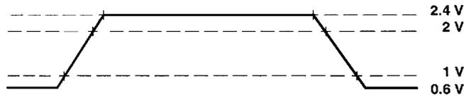
Figure 2. TTL-Level Outputs
