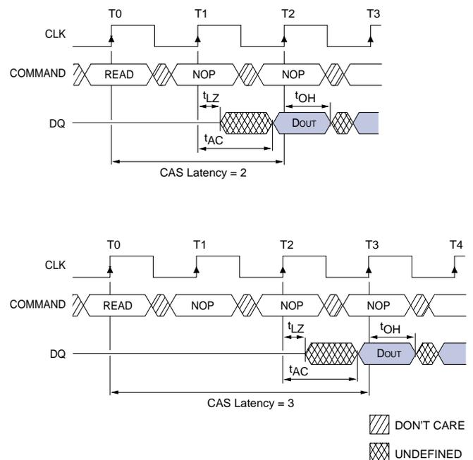
before the clock edge at which the last desired data element is valid, where  $x$  equals the CAS latency minus one. This is shown in Figure 7 for CAS latencies of two and three; data element  $n + 3$  is either the last of a burst of four or the last desired of a longer burst. The 64Mb SDRAM uses a pipelined architecture and therefore
