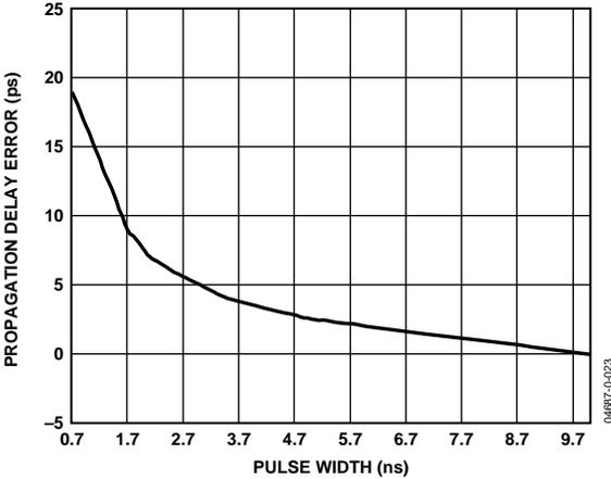
Figure 16. Propagation Delay Error vs. Pulse Width
