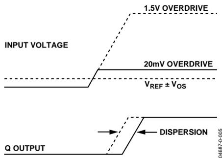
Figure 19. Propagation Delay Dispersion
