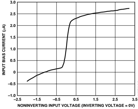
Figure 6. Input Bias Current vs. Input Voltage
