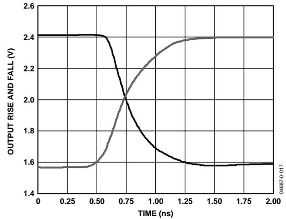
Figure 10. Rise and Fall of Outputs vs. Time
