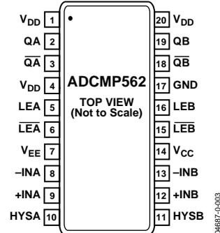
Figure 5. ADCMP562 20-Lead QSOP Pin Configuration
