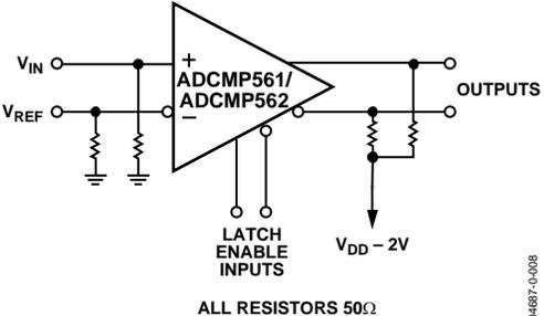
Figure 22. High Speed Sampling Circuits
