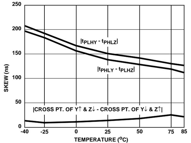
FIGURE 11. DRIVER SKEW vs TEMPERATURE (ISL8487, ISL81483)
