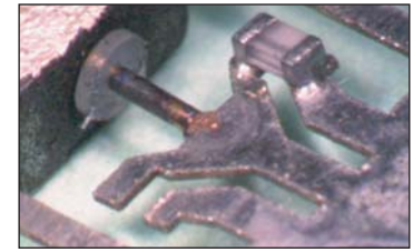
Anode, fuse and leadframe assembly
