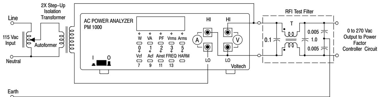
**Figure 25. Power Factor Test Set-Up**
