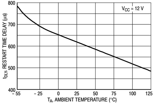
Figure 9. Restart Timer Delay versus Temperature
