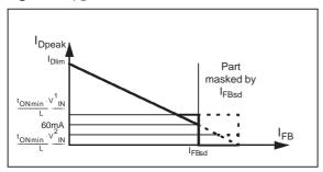
primary inductance value of the transformer and the input voltage. Two cases may occur, depending on the value of this current versus the fixed 60 mA, as described above.
