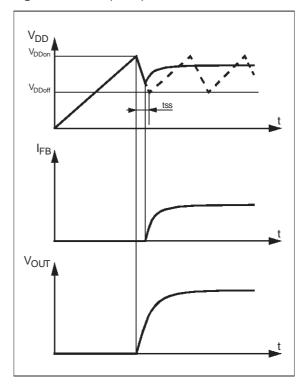
continuous supply. If the value of this capacitor is too low, the start up phase is terminated before receiving any energy from the auxiliary winding and the converter never starts up. This is illustrated also in the same figure in dashed lines.
