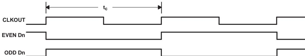
NOTE A: The worst-case test pattern produces the maximum switching frequency for all of the outputs.
