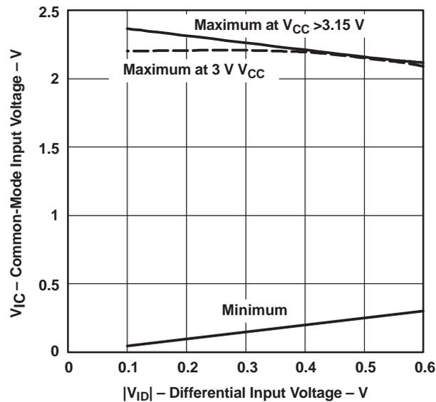
Figure 3. Common-Mode Input Voltage vs Differential Input Voltage
