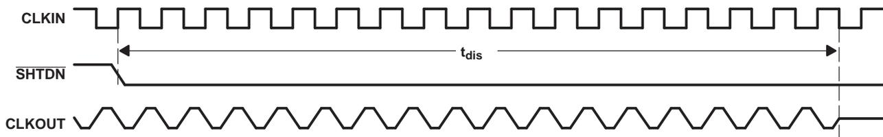
Figure 10. Disable Time Waveforms
