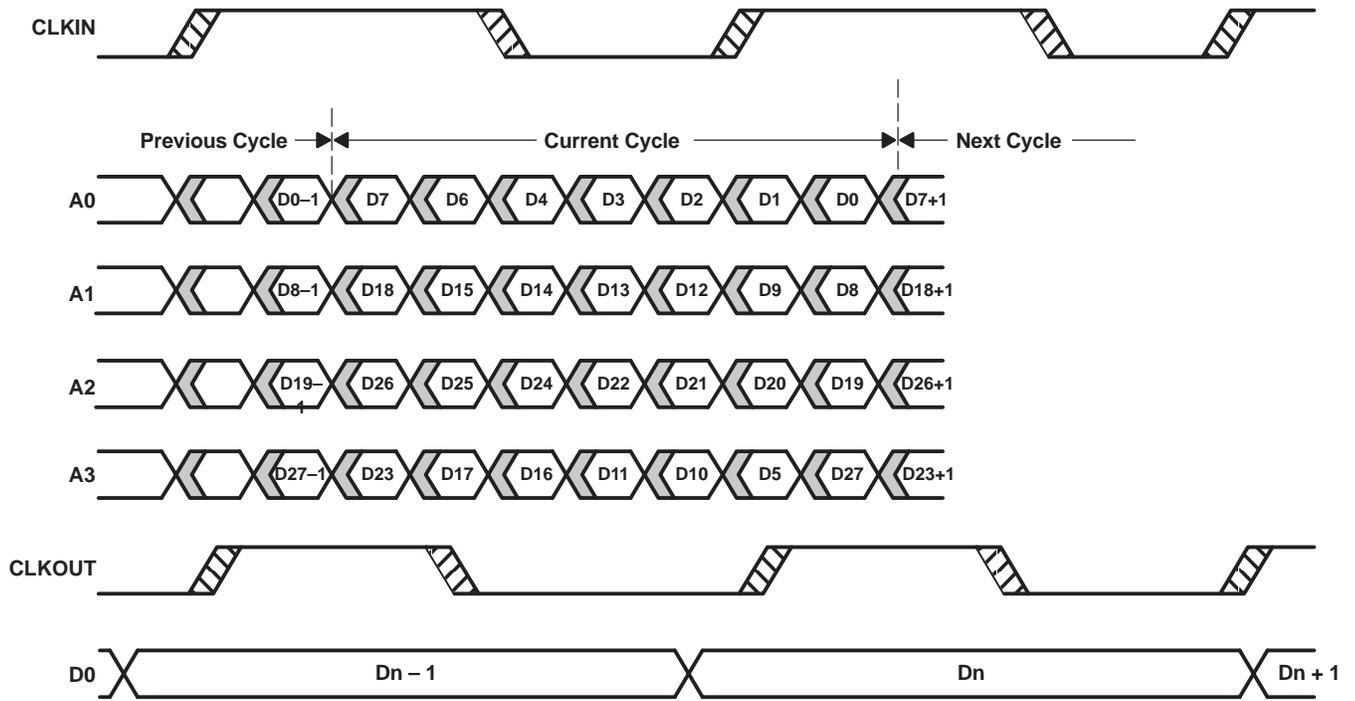
**Figure 1. SN75LVDS82 Load and Shift Timing Sequences**
