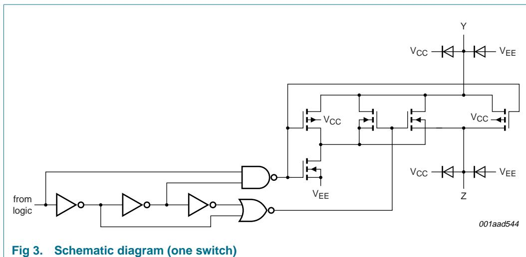
Fig 3. Schematic diagram (one switch)
