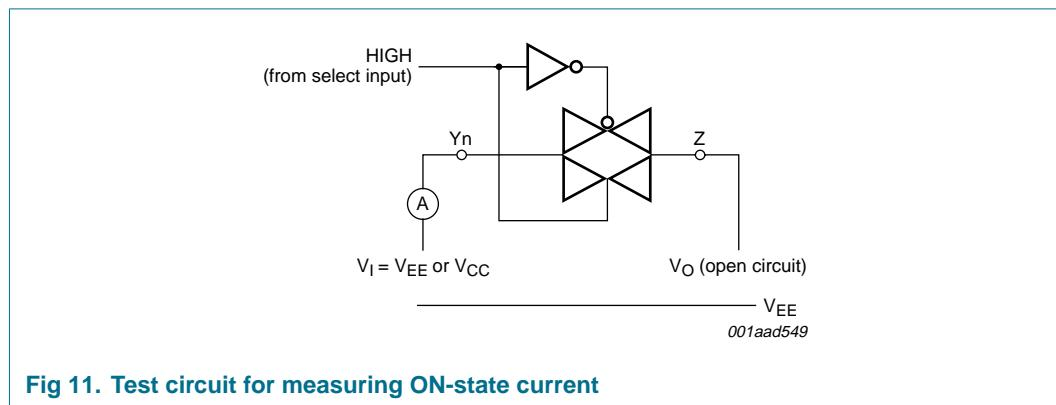
**Fig 11. Test circuit for measuring ON-state current**
