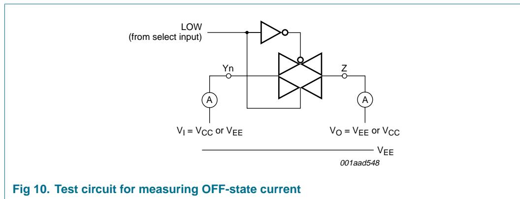
**Fig 10. Test circuit for measuring OFF-state current**
