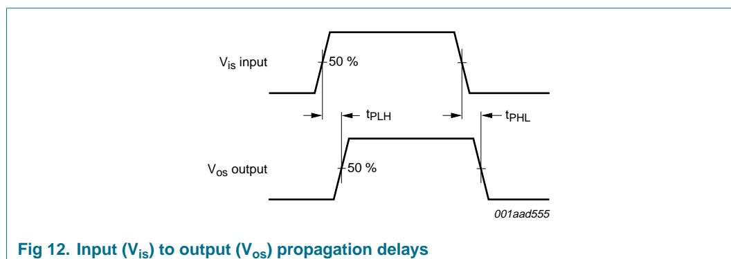
**Fig 12. Input ( $V_{IS}$ ) to output ( $V_{OS}$ ) propagation delays**
