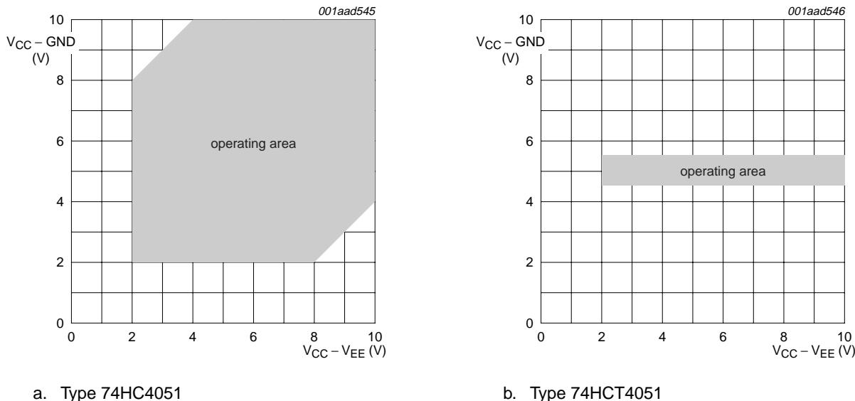
Fig 7. Guaranteed operating area as a function of the supply voltages
