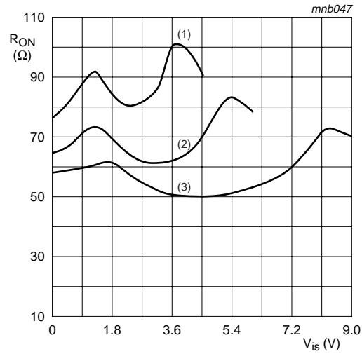
**Fig 9. Typical  $R_{ON}$  as a function of input voltage  $V_{IS}$**
