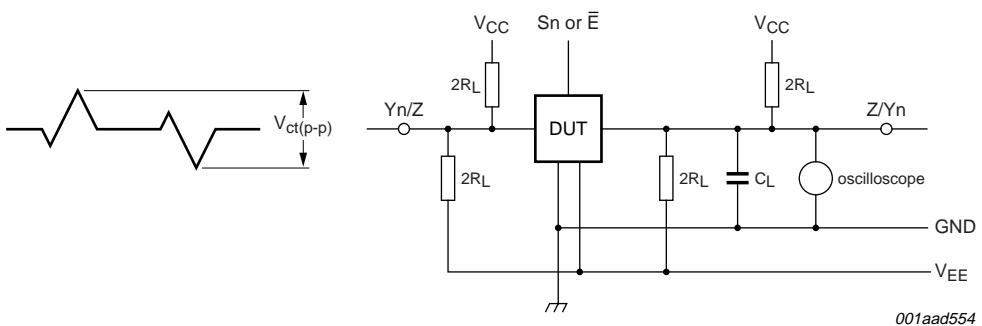
The crosstalk resembles the oscilloscope output shown in the left-hand drawing above.
