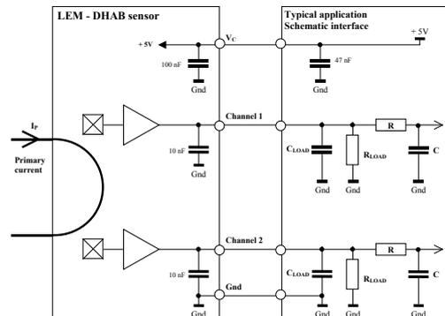
$R_L > 10 \text{ k}\Omega$  optional resistor for signal line diagnosis
