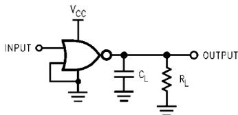
C<sub>L</sub> includes load and stray capacitance
