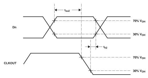
Figure 6. Setup and Hold Time Waveforms
