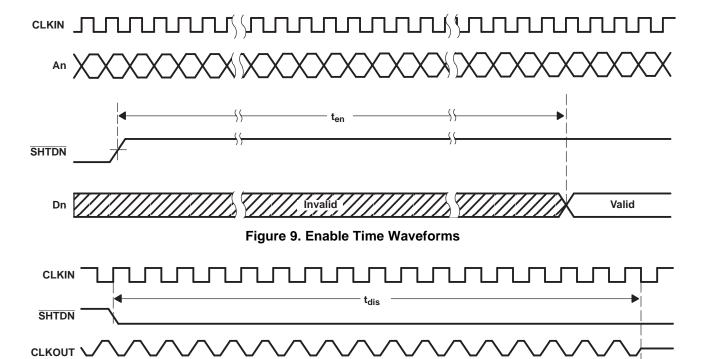
Figure 10. Disable Time Waveforms
