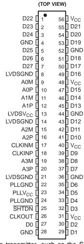
These functions allow receipt of synchronous data from a compatible transmitter, such as the SN75LVDS81, over five balanced-pair conductors, and expansion to 28 bits of single-ended low-voltage TTL (LVTTL) synchronous data at a lower transfer rate. The SN75LVDS82 can also be used with the SN75LVDS84 or SN75LVDS85 for 21-bit transfers.
