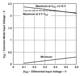
Figure 3. Common-Mode Input Voltage vs Differential Input Voltage
