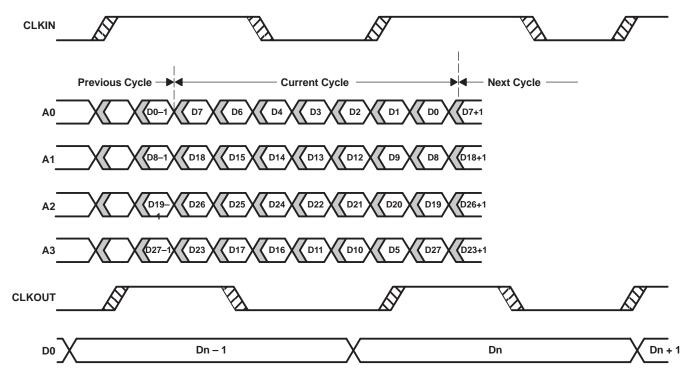
Figure 1. SN75LVDS82 Load and Shift Timing Sequences
