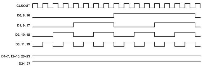
NOTE A: The 16-grayscale test-pattern tests device power consumption for a typical display pattern.
