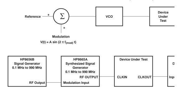
Figure 8. Input Clock Jitter Test
