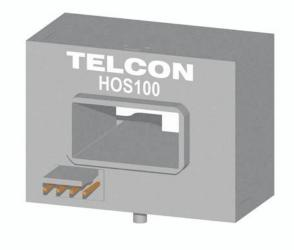
The HOS series are Open Loop Hall Effect Current Transformers covering the range of 100A to 600A. The product provides a voltage output which is galvanically isolated from the primary conductor. Designed to be panel mounted, or strapped to a bus bar the HOS series is controlled via an industry standard connector.
