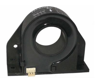
The HOL series are Open Loop Hall Effect Current Transformers covering the range of 100A to 1000A. The product provides a voltage output which is galvanically isolated from the primary conductor. Designed to be panel mounted, the HOL series is controlled via an industry standard connector.
