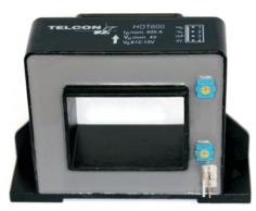
The HOT series are Open Loop Hall Effect Current Transformers covering the range of 100A to 1500A. The product provides a voltage output which is galvanically isolated from the primary conductor. Designed to be panel mounted, or strapped to a bus bar the HOT series is controlled via an industry standard connector.
