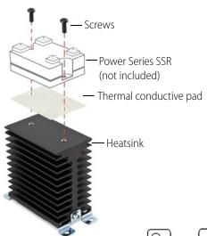
NOTE: To take advantage of the cooling effect of natural air flow, mount the SSR/heatsink assembly to a vertical surface with the Opto 22 logo right side up as shown here.
