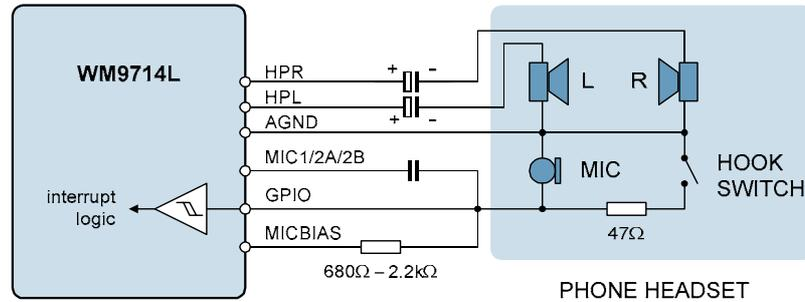
**Figure 36 Hookswitch Detection Circuit**
