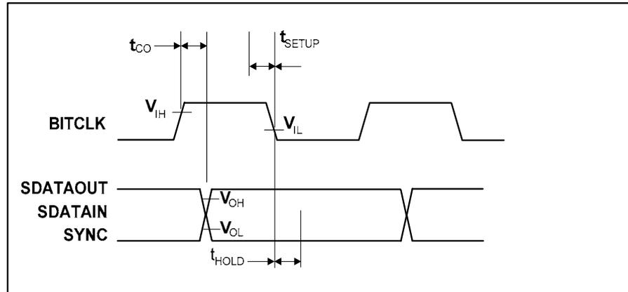
Figure 2 Data Setup and Hold (50pF External Load)
