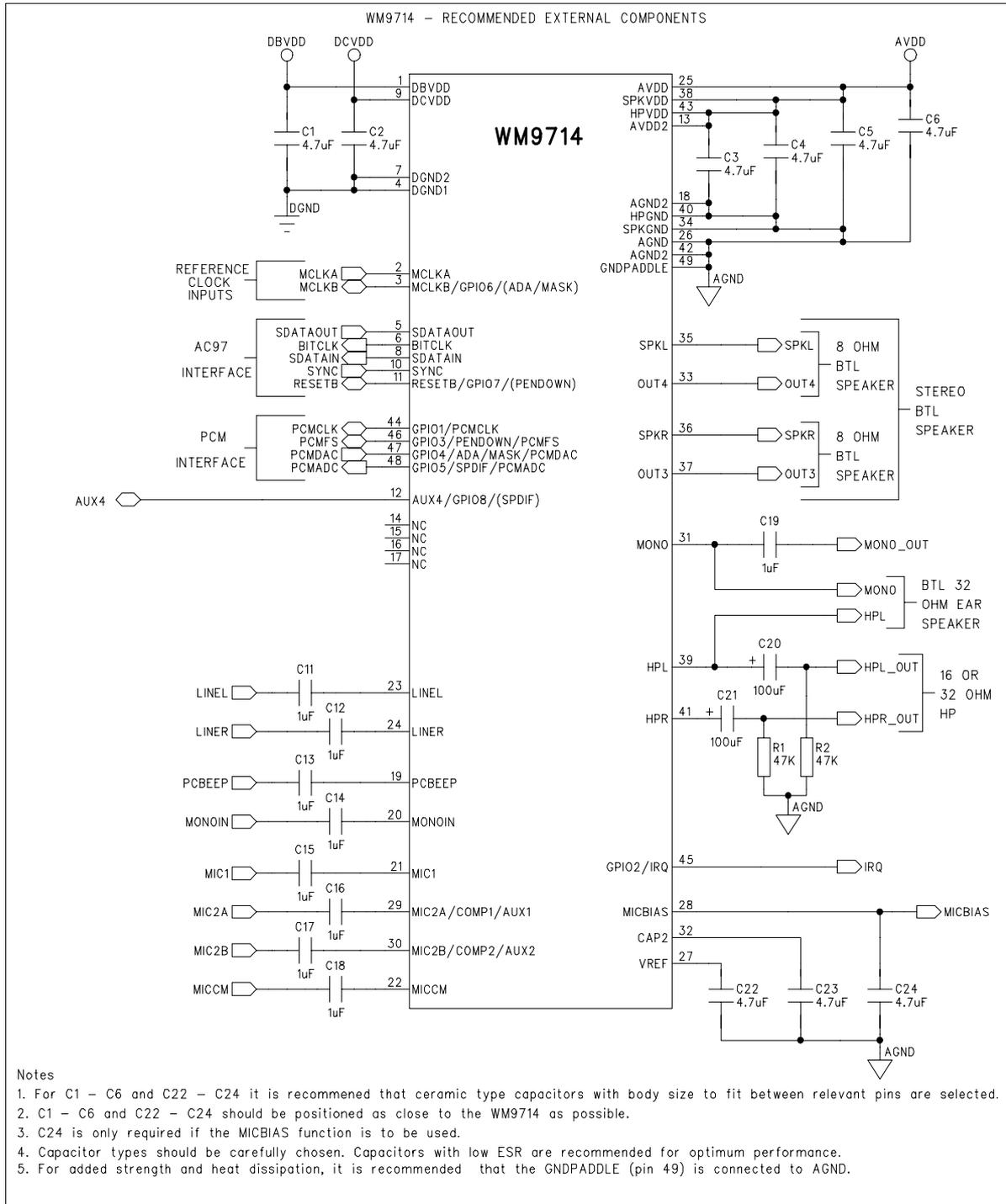
Figure 28 Recommended External Component Diagram
