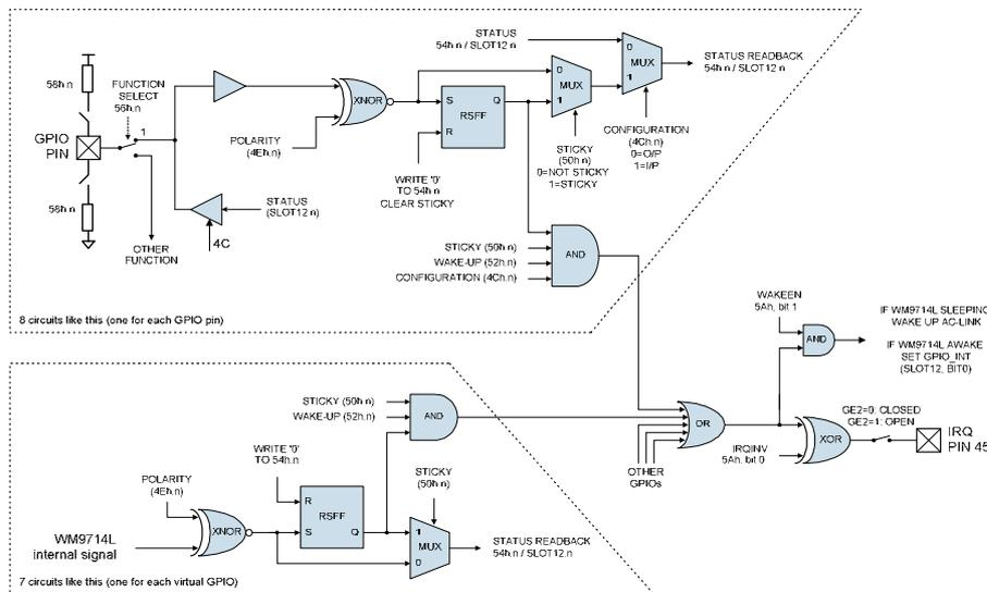
Figure 27 GPIO Logic
