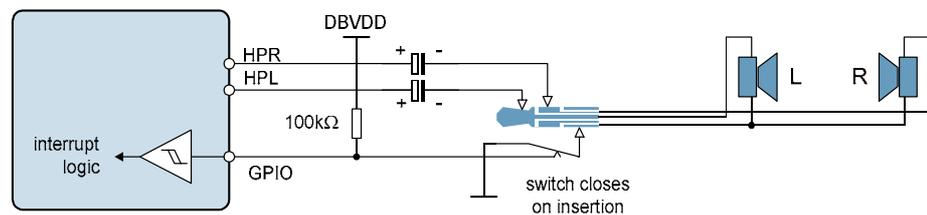
Figure 35 Jack Insert Detection Circuit
