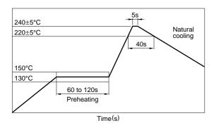
RECOMMENDED REFLOW SOLDERING CONDITIONS
