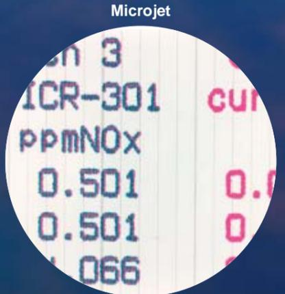
The ink jet printing mechanism allows continuous recording for a maximum of 12 channels (6 channels with 100mm width recorder) in 6 different colors. An A/D converter is used for each input signal for high speed data sampling to obtain a trace similar to that obtained by conventional pen mechanism recorders. Digital printing is also possible in the same color as the channel color, so clear and visible recording can be obtained. (for model PHA, PHC)
