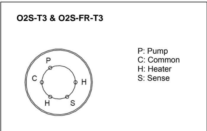
For detailed information on the sensor operation please refer to the following application note: AN0043 Operation Principle and Construction of Zirconium Dioxide Oxygen Sensor.
