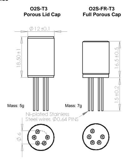
NOTE: Sensor pins are NOT designed to be solder too. Preferred method of connection is to crimp onto pins.
