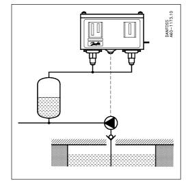
In a hydrophore system where water is pumped from a well or an open tank, both bellows are connected to a pressure outlet on the air side in the pump pressure line, if possible.
