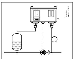
In a booster system receiving pressurized water the righthand bellows is connected - to the low pressure side of the pump for
