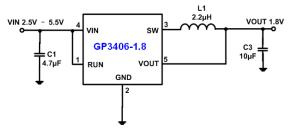
Figure 4. Basic Application Circuit with fixed output versions
