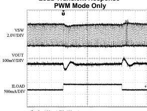
Iload = 100 mA TO 400 mA L=2.2uH, Cin=10uF, Cout=10uF, Vin=3.6V, Vout=1.8V
