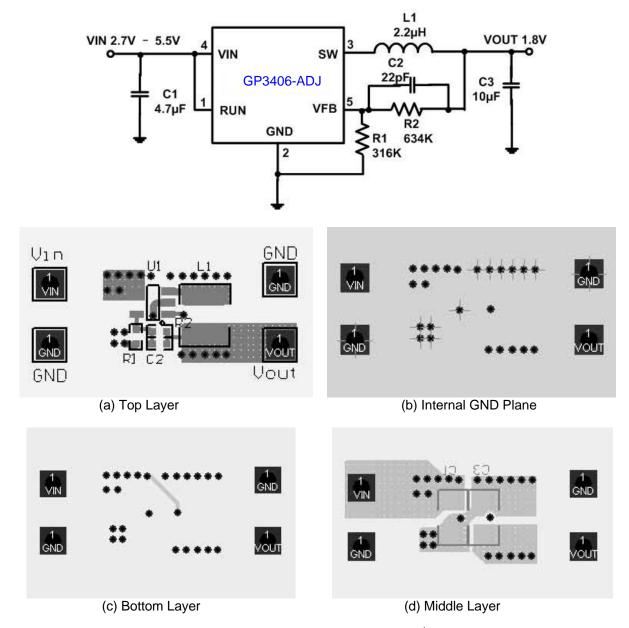
Figure 3. GP3406 Four Layers Layout Example, with the 2 nd and 3rd Internal Plane GND
