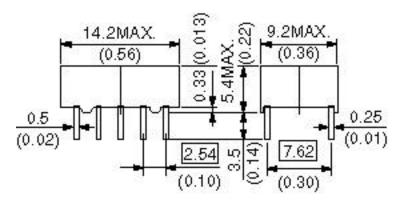
Note: Tolerance ±0.2 unless otherwise specified NJ: Cover hight — 6.25mm, Lead —2.8mm
