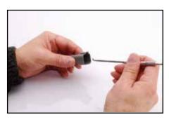
1. Remove wedge by inserting a hook into an opening of the wedge.
