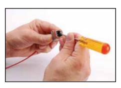
3. Use the same flathead screwdriver to remove contact inside connector.
