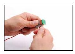
2. Twist the flathead screwdriver until wedge 'pops' out of connector.
