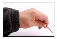
1. Grasp crimped contact approx. one inch behind the contact barrel.
