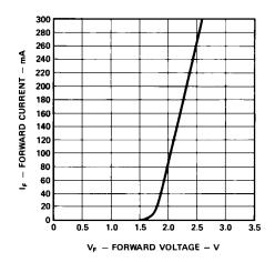
Figure 2. Forward current vs. forward voltage.
