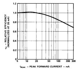
Figure 4. Relative efficiency vs. peak forward current.
