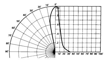
Figure 9. Relative luminous intensity vs. angular displacement. HLMP-D105.
