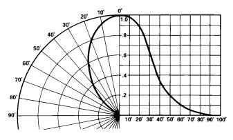
Figure 7. Relative luminous intensity vs. angular displacement. HLMP-D101.
