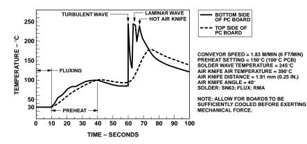
Figure 11. Recommended wave soldering profile.
