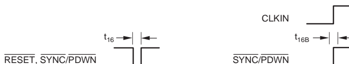
Figure 3. \overline{\text{RESET}} and \overline{\text{SYNC/PDWN}} Timing
