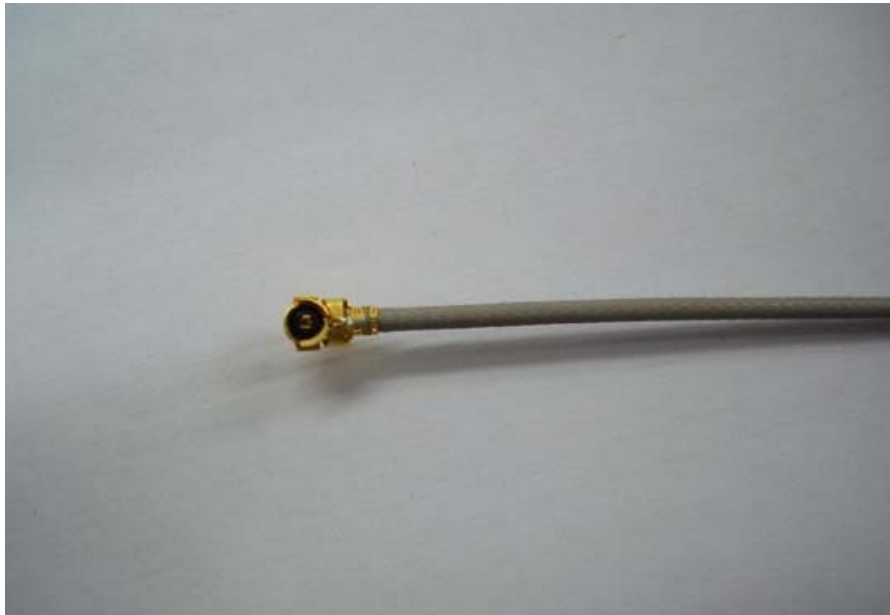
4) I-PEX MHF OD1.37mm Series Cable Assembly (20351-111R-37) :
