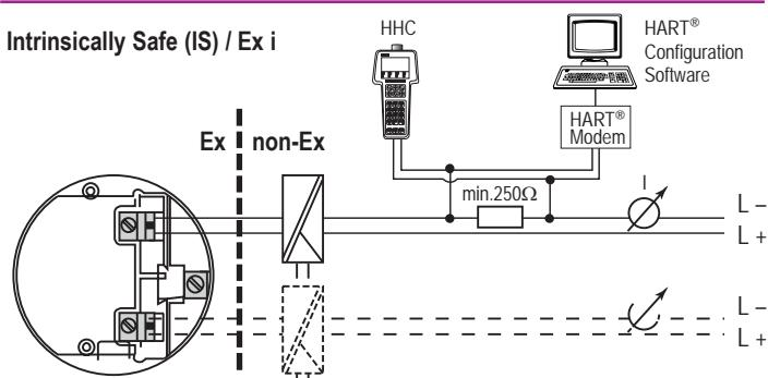
**Note:** Other options how to connect the HHC (Hand Held Communicator) and modem to the HART® loop are available.
