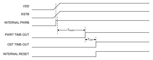
Note:  $T_{PWRT} = 18 \text{ ms}$ ;  $T_{OST} = 128 \text{ oscillator cycle time}$
