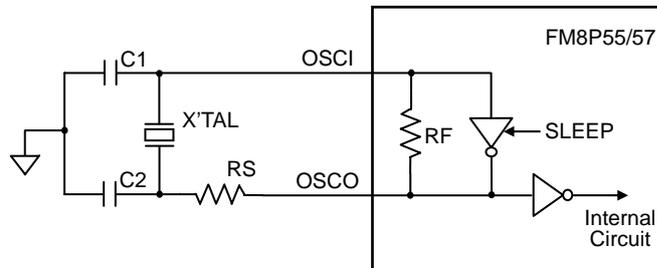
**FIGURE 2.9: HF, XT or LF Oscillator Modes (External Clock Input Operation)**
