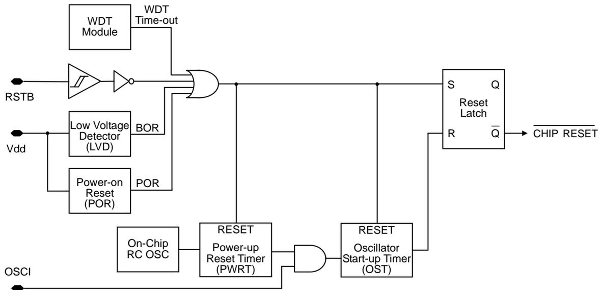
**FIGURE 2.6: Time-out Sequence on Power-up (RSTB Pin Tied to Vdd)**
