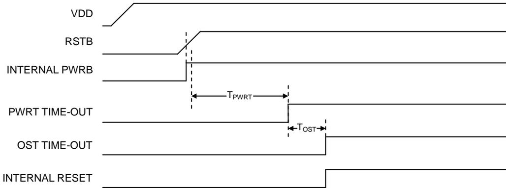
Note:  $T_{PWRT} = 18 \text{ ms}$ ;  $T_{OST} = 128 \text{ oscillator cycle time}$
