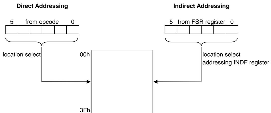
**FIGURE 2.2: Direct/Indirect Addressing for FM8P57/57E**
