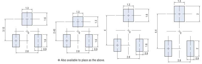
Note) The zero point is the center of mounting.
