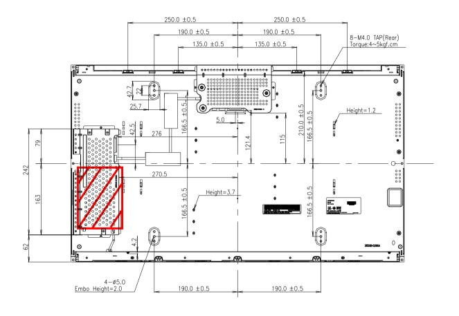
NOTES 1.UNSPECIFIED TOLERANCES TO BE  $\pm 0.5$ MM 2.TILT AND PARTIAL DISPOSITION TOLERANCE OF DISPLAY AREA ARE AS FOLLOWING. (1) Y-DIRECTION: | A-B |  $\leq 1.5$ (2) X-DIRECTION: | C-D |  $\leq 1.5$ BEZEL OPEN ACTIVE AREA
