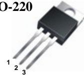
1.Gate 2. Drain 3. Source
