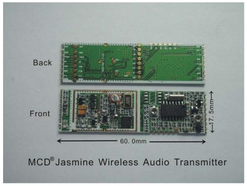
Notes: The highest part of MCD® Jasmine receiver is 11mm, and that of MCD® Jasmine transmitter 5.5mm.
