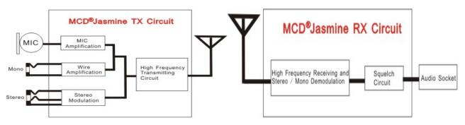
Application area: Wireless audio transmission with low cost and short-distance (300m in open space), such as amplifiers, lights of built-in speakers and teaching devices.
