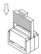
(2) Pull the removal key up to remove the module.
