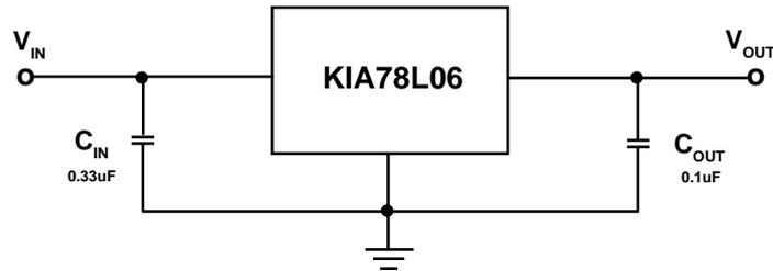
Note1: The input voltage must remain typically 1.7V above the output voltage.
