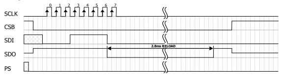
Figure 4: Reset command sequence SPI mode 0
