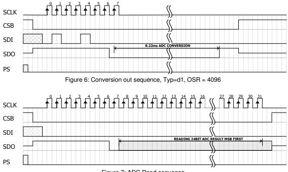
Figure 7: ADC Read sequence
