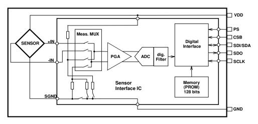
Figure 1: Block diagram of MS5605-02BA
