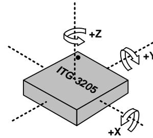
**Orientation of Axes of Sensitivity**
