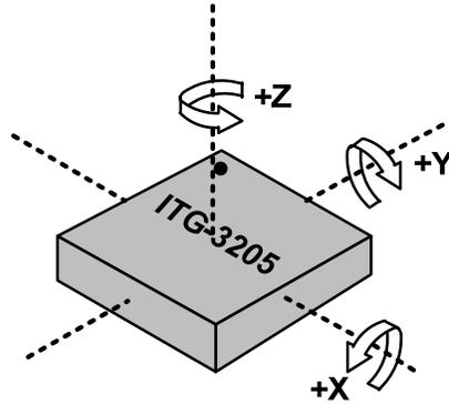
**Orientation of Axes of Sensitivity
