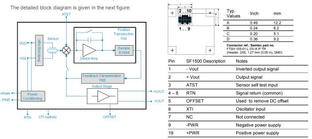
For the SF1500SN.A, the external oscillator should have the following specifications: 4.000MHz or 4.096MHz square wave output with 50% (range 40-60%) duty cycle and a 5V CMOS level voltages (low < 0.8V, high >4V). Note: do not apply XTI prior to applying both positive and negative power supply voltages.
