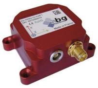
The IG-500N is a miniature and high performance GPS enhanced Attitude and Heading Reference System (AHRS). With its embedded Extended Kalman Filter, the IG-500N delivers unmatched precision for attitude and position measurements even during very high dynamic conditions.
