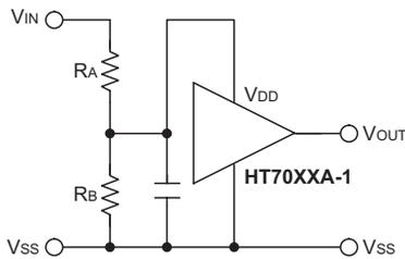
$$\text{Detectable voltage} = \frac{R_A + R_B}{R_B} \times V_{DET}$$
