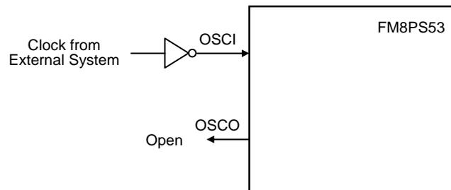
**FIGURE 2.8: ERC Oscillator Mode (External RC Oscillator)**
