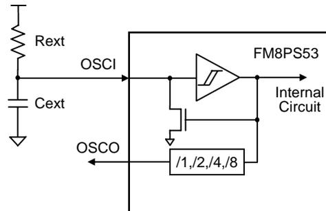
**FIGURE 2.9: ERIC Oscillator Mode (External R, Internal C Oscillator)**
