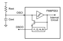
FIGURE 2.9: ERIC Oscillator Mode (External R, Internal C Oscillator)
