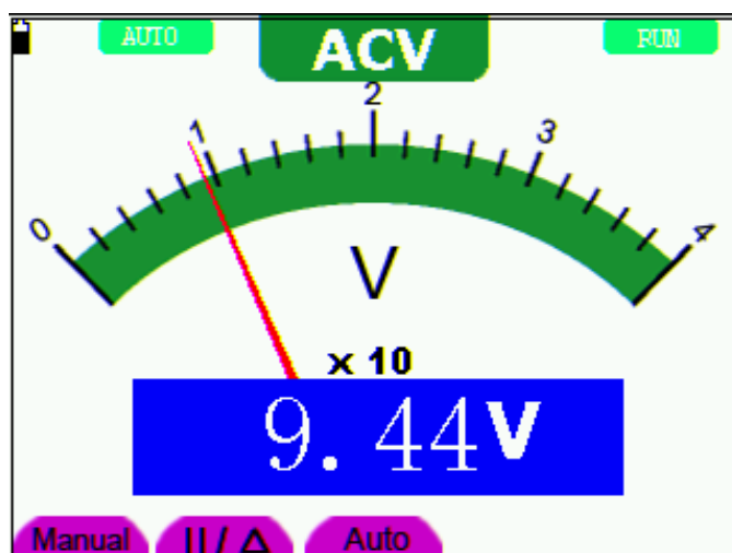
Figure 26: AC Voltage Measurement
