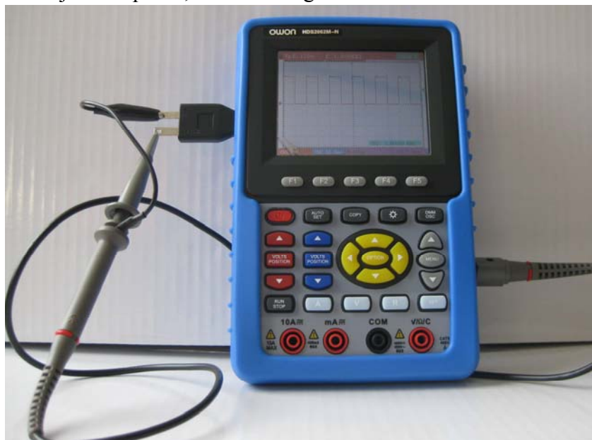
Fig.3. The connection of Square-wave test signal
