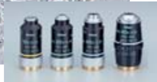
ADL objectives for Apodized phase contrast
