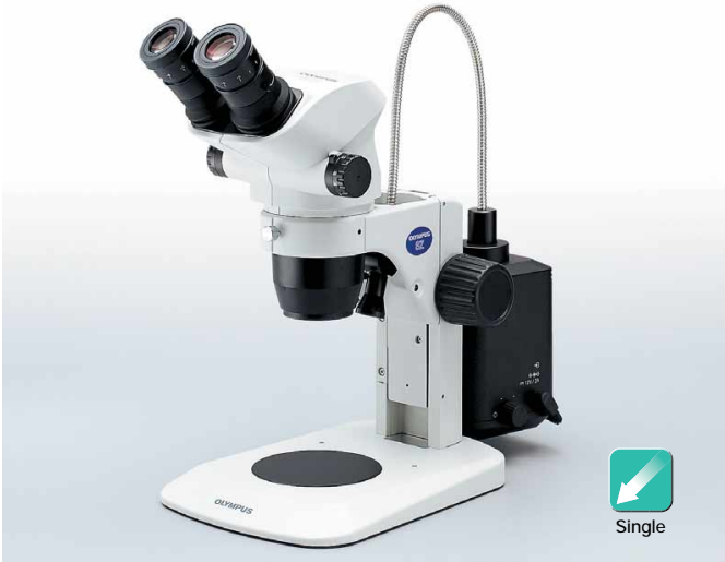
Flexible light guide / SZ2-LGSF A single fiber optic guide is fixed at the back of the objective so as not to disturb microscope operation.
