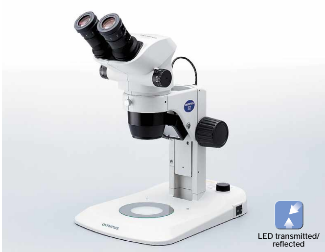
LED illuminator stand / SZ2-ILST The world's first LED stand features a thin design to keep sample positions low and to optimize operability. Simultaneous transmitted and reflected light are available on this stand. LED light offers both long lifetime and constant color temperature at any intensity.
