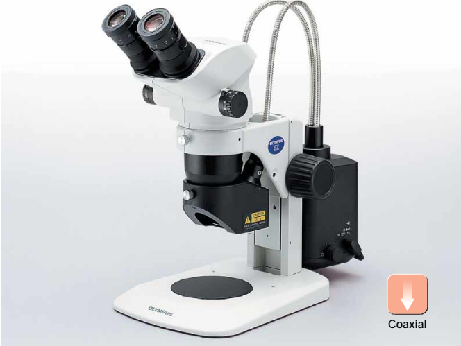
Coaxial reflected light illuminator / SZ2-ILLC It combines a polarizer and a 1/4λ plate, for easier viewing of specimens which are difficult to examine under oblique reflected light illumination.
