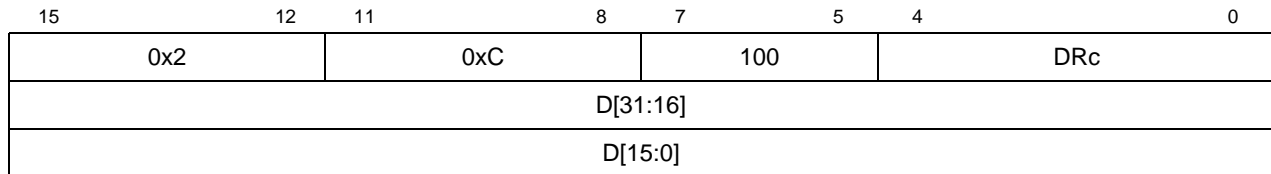
Figure 30-39. WDMREG BDM Command Format
