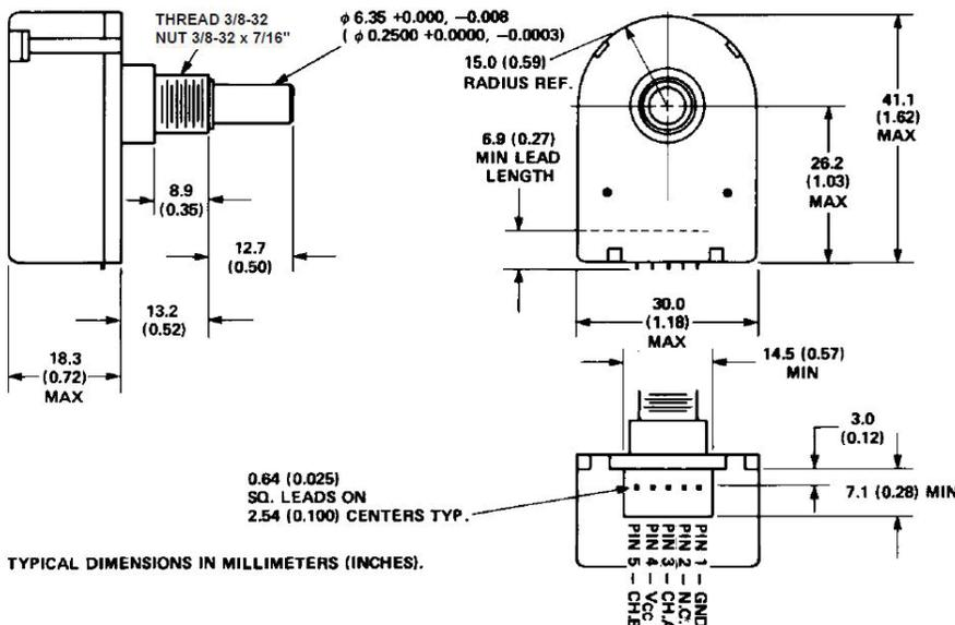
TYPICAL DIMENSIONS IN MILLIMETERS (INCHES).
