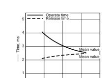
80 100 120 — Coil applied voltage, %V 4-(1) Influence of adjacent mounting Tested sample: DS2Y-S-DC12V, 10 pcs. Ambient temperature: 20°C 68°F
