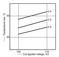
2-(2) Coil temperature rise 2 coil latching Tested sample: DS2Y-SL2-DC12V, 5 pcs. Measured portion: Inside the coil Ambient temperature: 21°C to 25°C 70°F to 77°F
